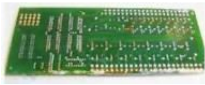
Untreated circuit board. Sprayed with salt water for ten days, significant oxidation noted.
